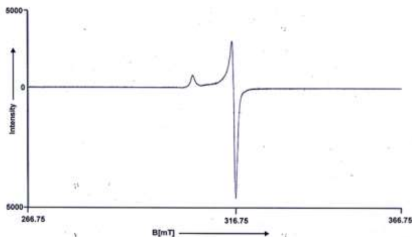
Figure 2: ESR of Bis(O-isobutyldithiocarbonato)(3-hydroxypyridine)copper(II).
