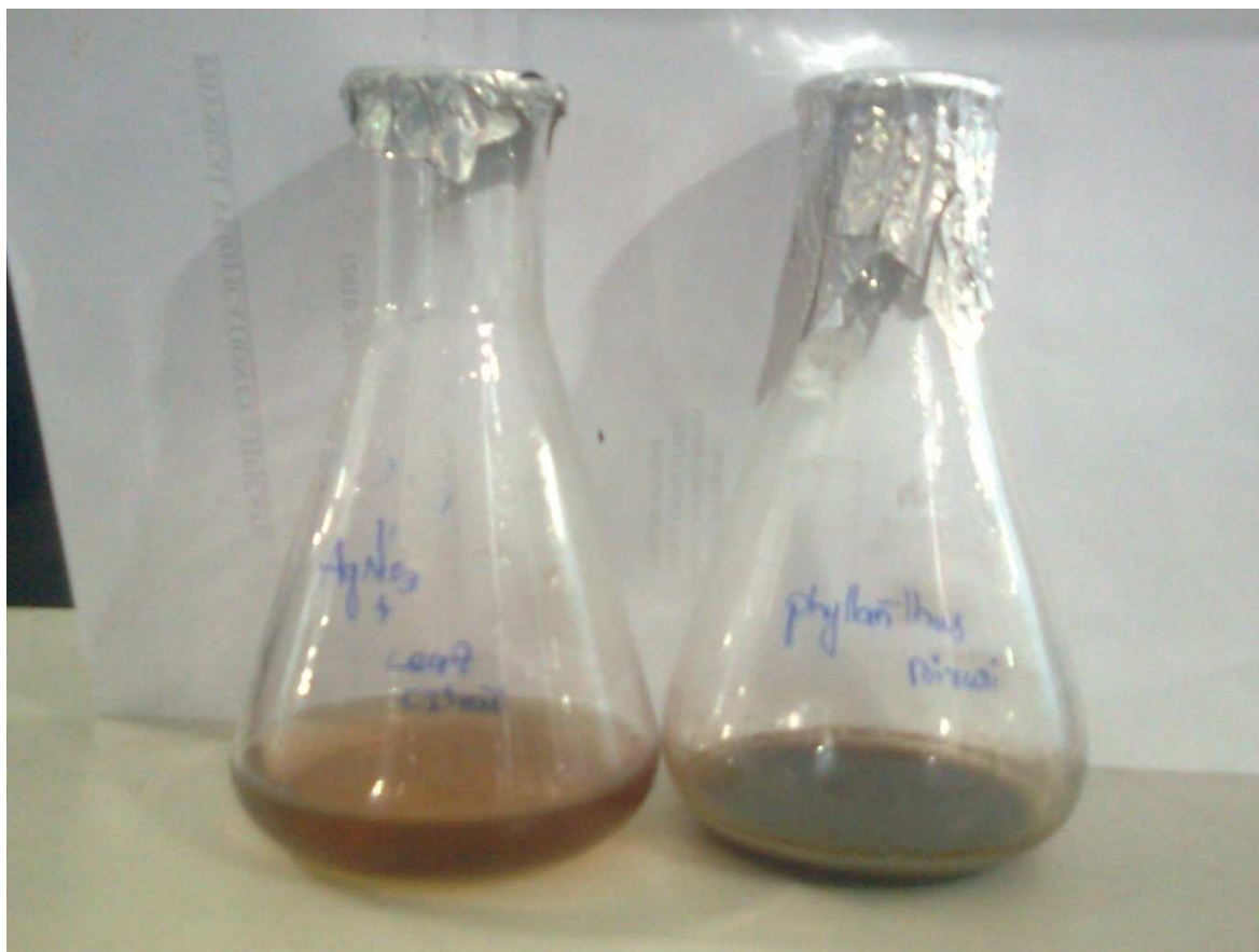
Fig 1: A) Green colour shows ethanolic extract of Phyllanthus niruri leaf. B) Brown colour shows the silver nanosolution.
