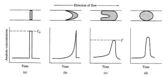
Fig 2: Effect of convection on concentration profiles of analytes at the detector, (a) no dispersion, (b) dispersion by convection, (c) dispersion by convection and radial diffusion, (d) dispersion by diffusion.
