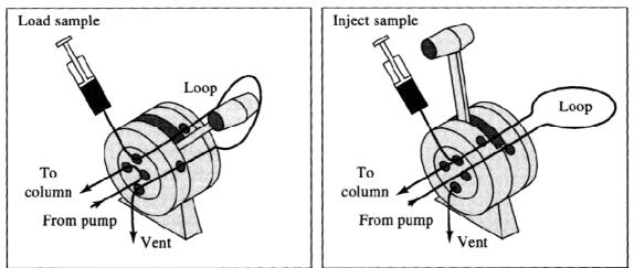
Fig 4: An injection valve
