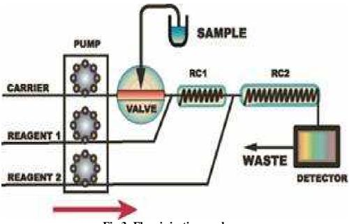
Fig 3: Flow injection analyzer
